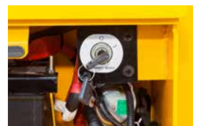
Battery master switch
