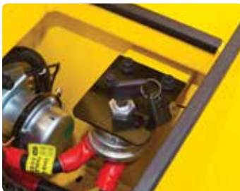
Master Switch A master switch disconnects the battery power to protect the electrical system from excess electrical drainage.
