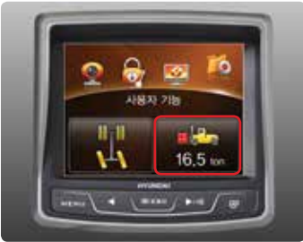
Load Indicator A load can be placed on the fork and can be accurately weighed by measuring the hydraulic pressure.
