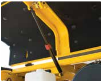
Automatic Self Locking Gas Spring Engine compartment hood is safely opened by a self locking gas spring.
