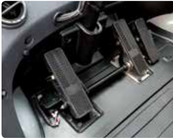
Ergonomically Positioned Pedals Based on human engineering the accelerator, brake and inching pedals are optimally positioned for the operator's convenience.
