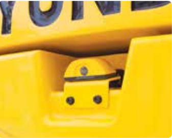
Rear View Camera The rear view camera makes the operation more easy and convenient. And it supports 4 camera channels.
