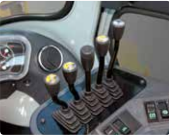
Quick Response of Operating Control Levers Only minimal operator's effort is required for precise, safe and productive control. (5-Lever, 6-Function : Standard) (5-Lever, 7-Function : Option)
