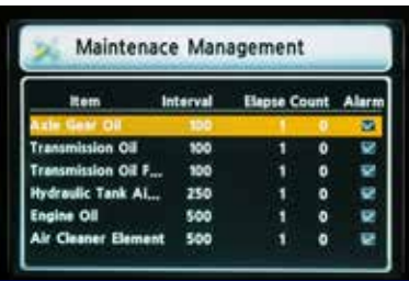
Maintenance management This indicator automatically alerts the operator of the replacement cycle of key consumable items.
