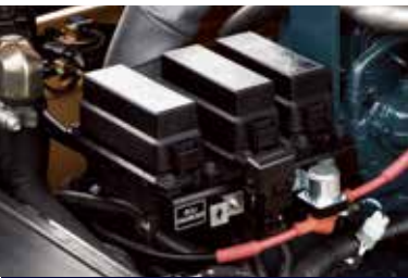
Waterproof & Dustproof cover Newly developed waterproof and dustproof fuse box and relay box for ease of maintenance.
