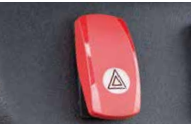
Emergency switch (OPT) A button-type switch enables to notify of emergency situations quickly.
