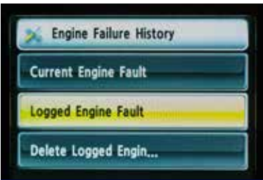
Engine fault diagnosis Details of engine fault diagnosed by the engine control unit (ECU) can be checked on the dashboard.
