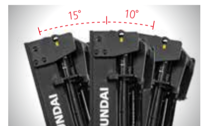
Mast Tilting Angle
